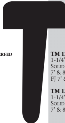
T-ASTRAGALS: AN ASTRAGAL, T-LIKE IN SHAPE, IS RABBETED TO THE APPROXIMATE THICKNESS OF THE SWINGING DOOR.
