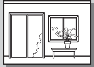
CASING: USED TO TRIM INSIDE AND OUTSIDE DOOR AND WINDOW OPENINGS.
